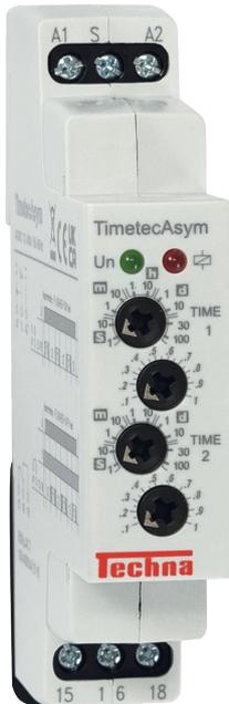
The TimetecAsym is a Cycling Timer with two independently adjustable time periods for on and off, and the choice of starting the cycle with the relay on or off. Each time cycle also has a scale of between 0.1s – 100 days divided between 10 time ranges, to allow for the most extreme of requirements.
